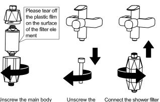
Unscrew the main body of the filter housing and take out the filter element
