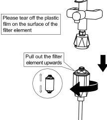
Open the lower cover of the filter case counterclockwise, take out the old filter, install the new filter element and tighten themain body of the filter case by rotating clockwise
